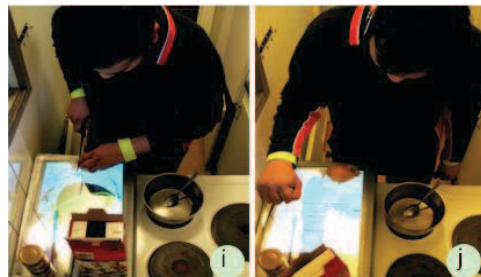
Fig. 2. A subject performing the physical-virtual activity of preparing breakfast where the cutting board smart object is used for cutting onions (i) and for accessing recipe information using speech and gestures (j).
