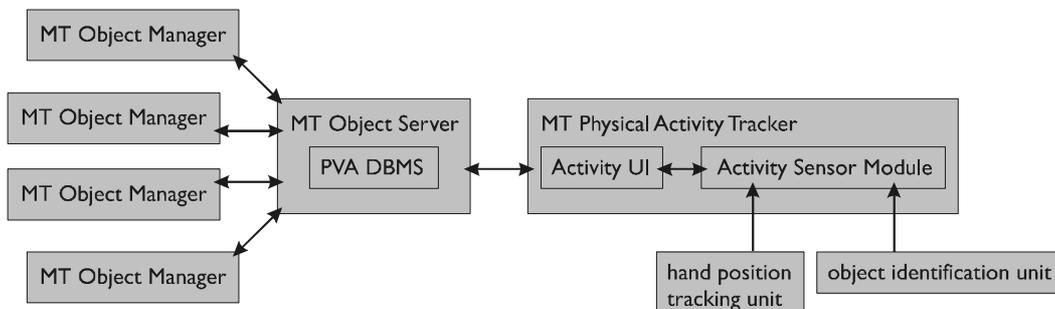
**Figure 5:** The basic Magic Touch system architecture consisting of (1) object managers providing special-purpose GUIs, (2) physical activity tracker clients handling input from sensors in a specific physical environment, and (3) an object server that keeps all authorised clients up-to-date with information about any alteration on Physical-Virtual Artefacts performed by users.
